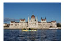
Launching its operation in September, the amphibious vehicle is the result of international cooperation. The hull, designed by a British naval engineer, was manufactured in Malta; the undercarriage and powertrain come from the Italian plant of IVECO; the jet engine is also Italian, made by Castoldi. Thermosol, a Hungarian company prepared the vehicle to meet European Union's strict quality and
