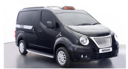
According to Nissan, the latest version will be adhering to the black cabs regulations set by the TfL which will be including a requirement of 25 feet or 7.6 meters of turning circle. TfL has licensed London's black cabs, traditionally called as Hackney Carriages. Also, the Licensed Taxi Drivers Associations has welcomed this new line of vehicles and said that it would reap more competition into the market.
