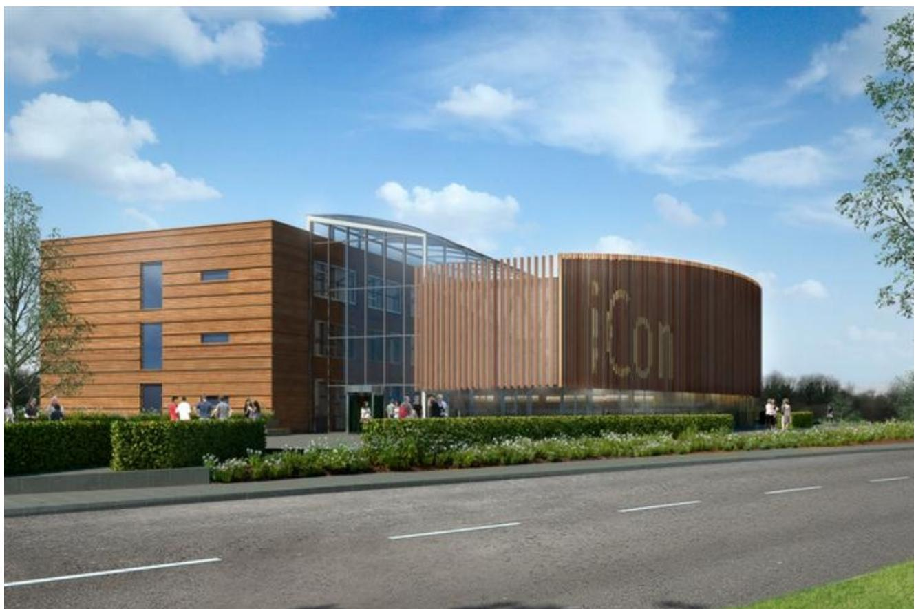
Located at the centre of England in Daventry, it is a well-connected base for any green and forward-thinking business. The building's low carbon design features include a natural ventilation system and panels in the ceiling that can absorb or emit heat, depending on the temperature. The roof is made of an inflatable plastic membrane, similar to the material used on the Eden project in Cornwall.
